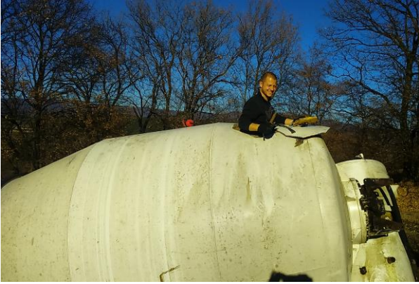
Fig. 4. Concrete mixer revision hole
