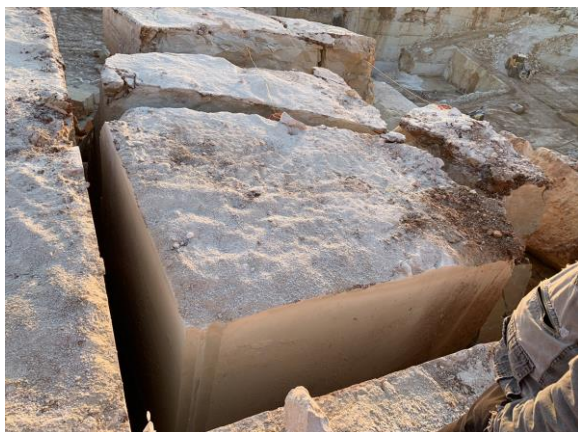
Fig.12. Effect of mechanical pre-cutting
