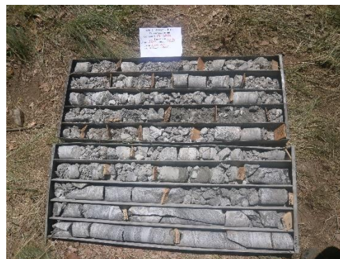
Fig. 1. Typical sequence of intact and crushed core intervals (depth interval 37m-47m).
