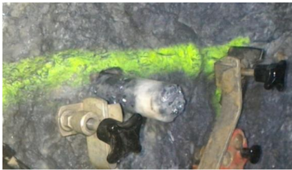
Fig. 2. Drilling core samples out of the host massif
