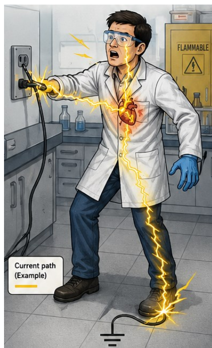
Fig 1. Short circuit on the human body
