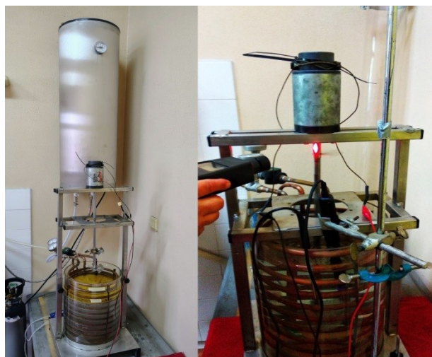
Fig. 5. Laboratory reactor in operating mode
