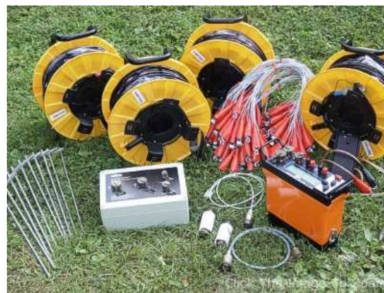
Fig. 4. Electrical resistivity equipment
