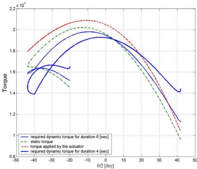
Figure 2 Static and dynamic torques at the second joint [N·m]
