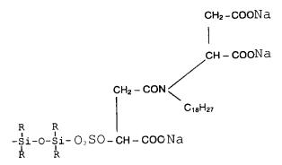
Hardening of the collector adsorbed along the borderline of liquid-gas-waters until easy disruption of the slime seams between the air bubbles, coalescence of the latter and disruption of the froth.
