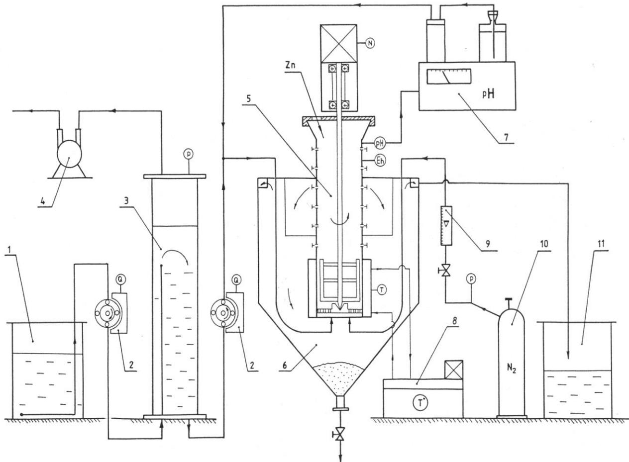
Figure 1. Batch-scale cementation installation
