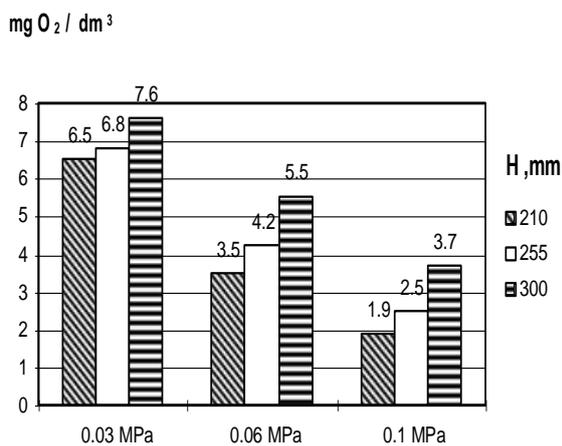
Figure 4. Dynamic of dissolved oxygen on different column high
