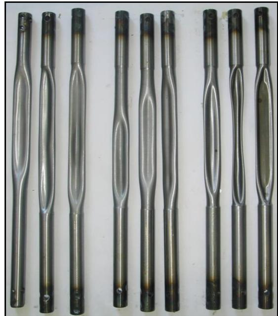
Fig. 11. Collapsed test specimens made of 10MoCr10 steel
