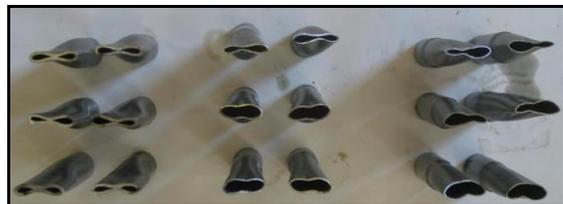
Fig. 12. Sectioned test specimens made of E235 steel
