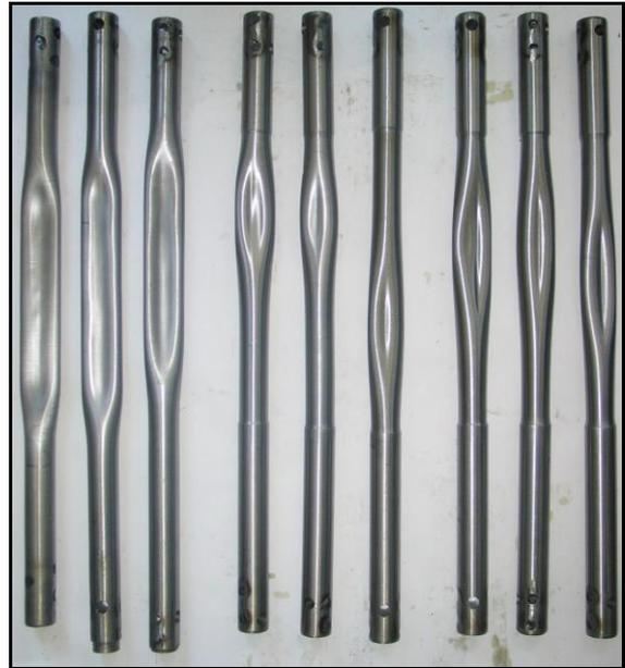
Fig. 10. Collapsed test specimens made of E235 steel
