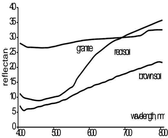
Fig. 1a. Reflectance spectra of granite, brown and red soils
