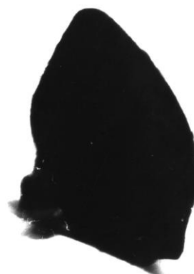
Figure 3. Zone of oxidation of copper and molybdenum and porphyritic deposits: molybdite, electronic microphotography, suspension, increased 30 400x
