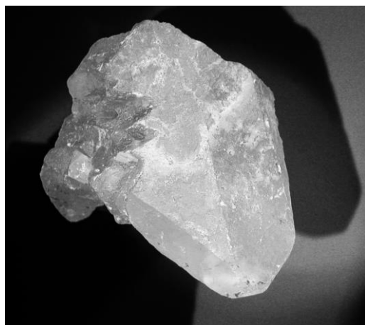
Figure 8. Calcite crystal, combination of scalenohedron (+) and (-), hexagonal prism and rhombohedron.
