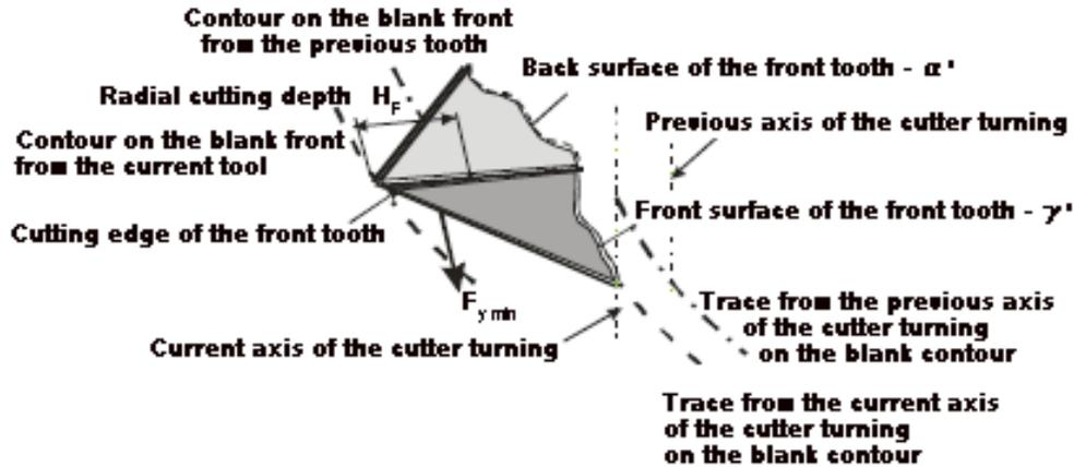
Fig. 8. Conical part of a shank cutter at a contour millicut-in
