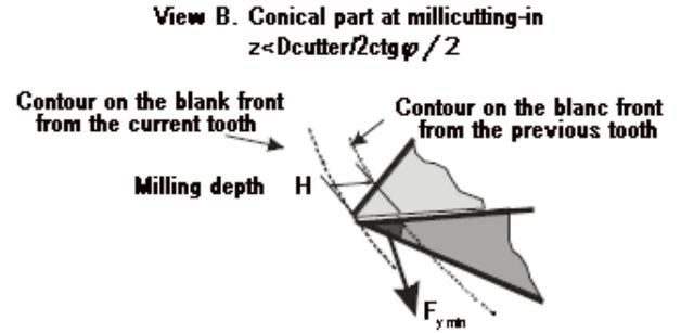
Fig. 7. Shank cutter at contour millicut-in
