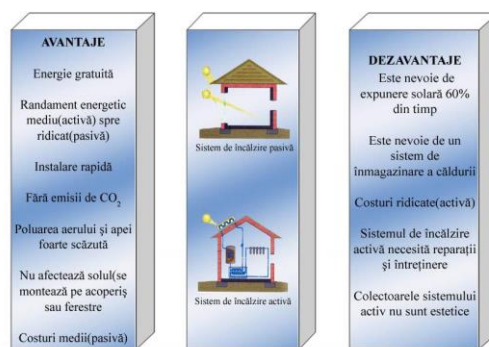
Fig. 2. Advantages and disadvantages for using active and passive solar energy for room-heating.
