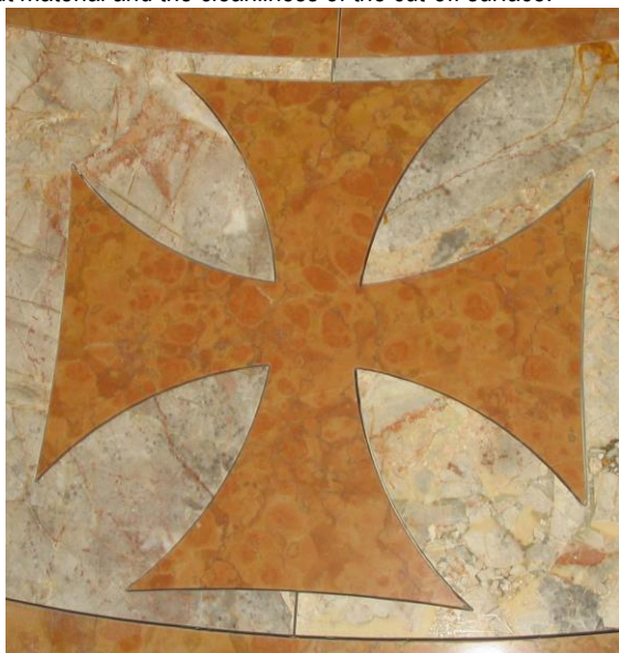
Fig. 11. Example of mosaics element, obtained bu water jet cutting.
