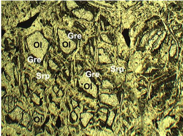
Fig. 7. The structure of the dunitic domains in which olivine (Ol) relics are surrounded by minerals of the serpentine group. The greenalite (Gre) is located exclusively near the olivine (Ol) relics. Here the iron from the serpentine group mineral is in the bivalent form (N|| 40x)
