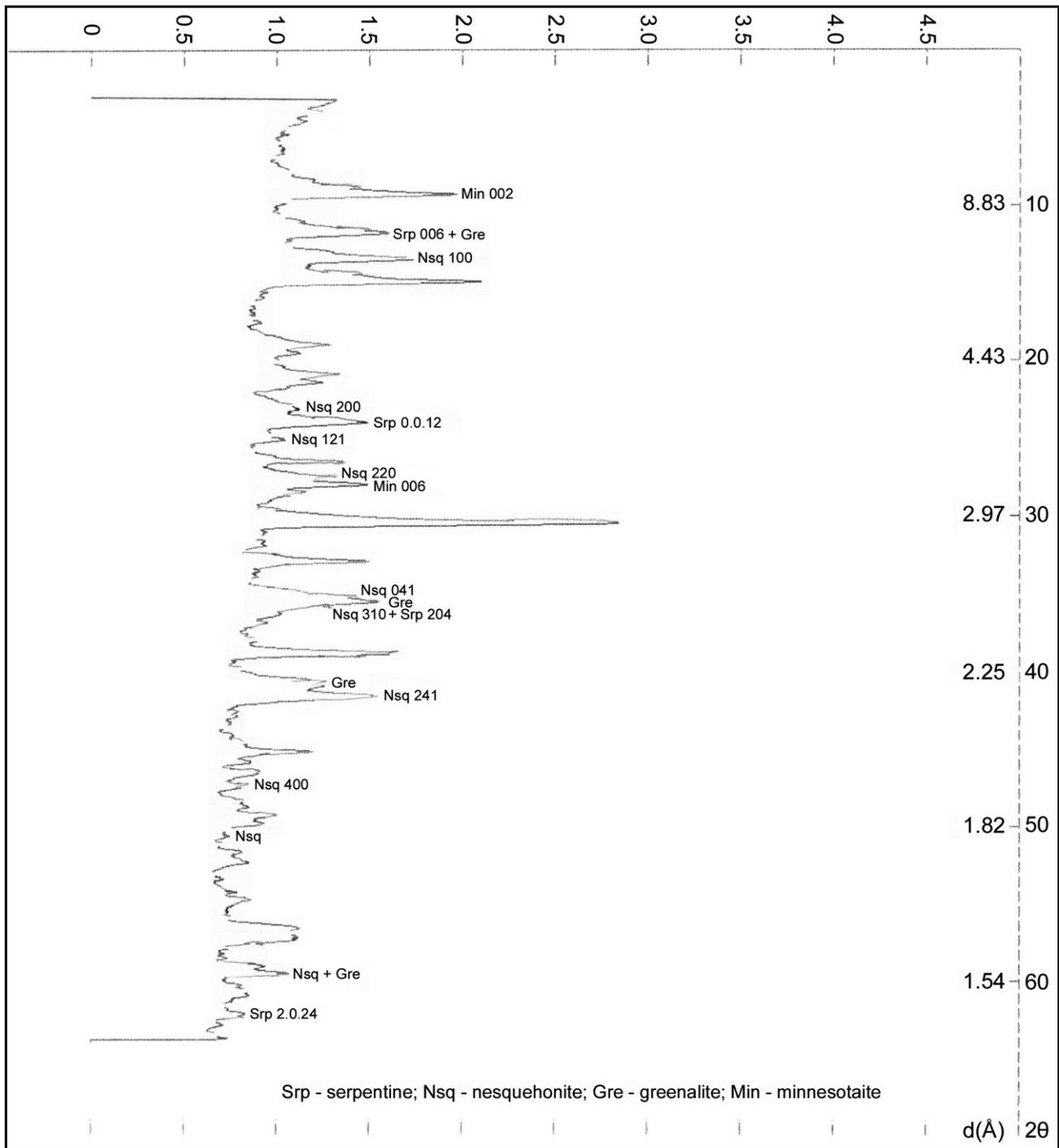
Fig. 9. Diffractogram of the sample from joints filling developed in ultrabasic massive from Tişovița
