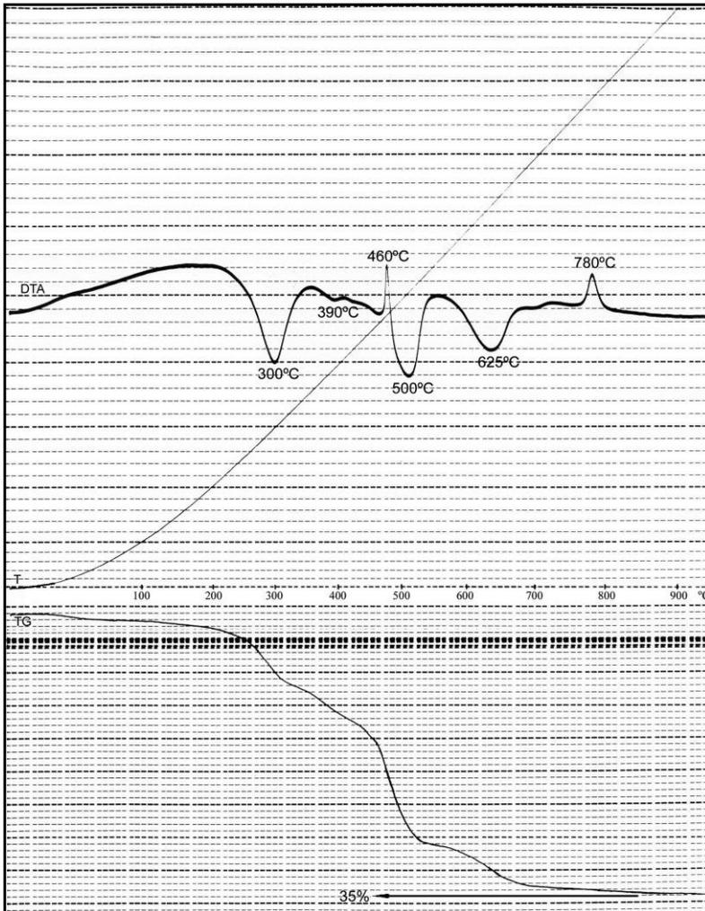
Fig. 10. Thermal derivatogram of the sample from joints filling developed in ultrabasic massive from Tişovița
