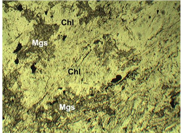
Fig. 6. The domains composed of colorless magnesian chlorite (Chl) and magnesite (N|| 40x)
