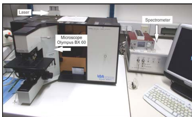
Fig. 1. Lasers "Raman" micro-spectrometer HORIBA in the Laboratory of fluid inclusions of the University of Leoben, Austria
