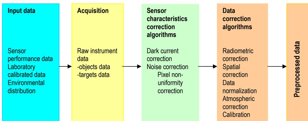
Fig. 2. Preprocessing data flow diagram
