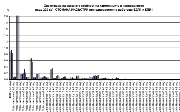
Fig. 6. Bar chart of the mean value of the voltage harmonics - 220 kV input – STOMANA INDUSTRY, EAF1 and LF1 operating in parallel
