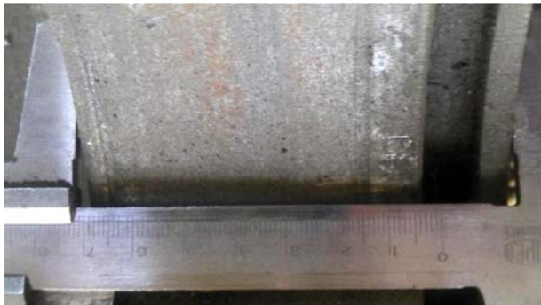
Fig. 2. Wear bearing housing
