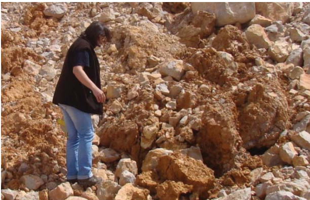
Fig. 3. Dilution. Mixing of pure limestone blocks with lumps of clay after the blasting so the clay cannot be separated from the limestone.
