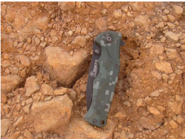
Fig. 1. Tectonized limestone from the Slivnitsa formation in West Bulgaria. Angular rock fragments are visible on the photograph, included in grinded mass with predominantly clay composition. In the absence of industrial washing installation this rock represent 100% loss from the reserves for production of products of higher technological grade.
