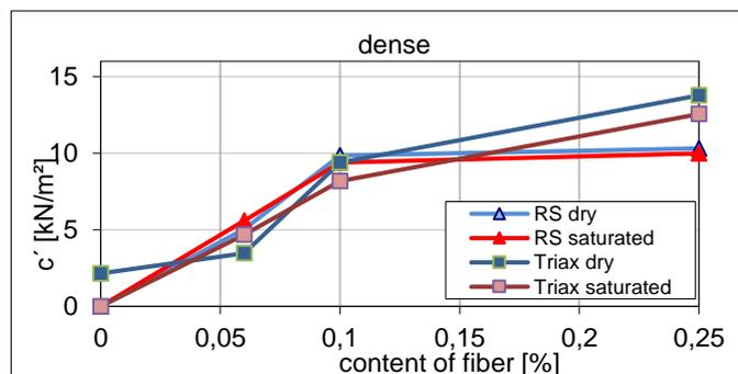
Fig. 7. content of fibre – cohesion (dense)
