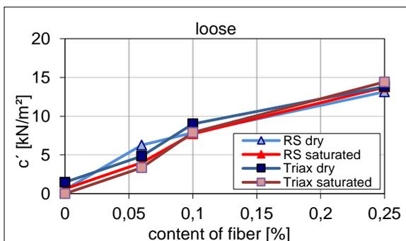
Fig. 6. content of fibre – cohesion (loose)
