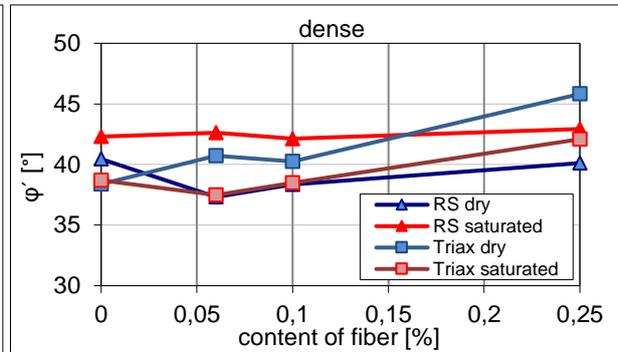
Fig. 7. content of fibre – friction angle  $\varphi$  (dense)
