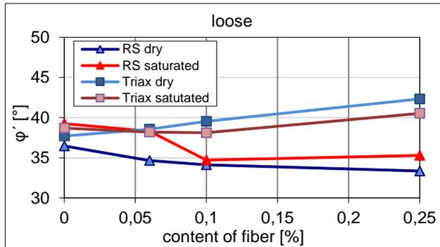
Fig. 6. content of fibre – friction angle  $\varphi$  (loose)
