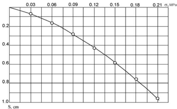
Fig. 6. Results of plate loading of the soil-cement cushion of the metal storehouse of the State Reserve in the town of Sindel (plate area – 24 m 2 )
