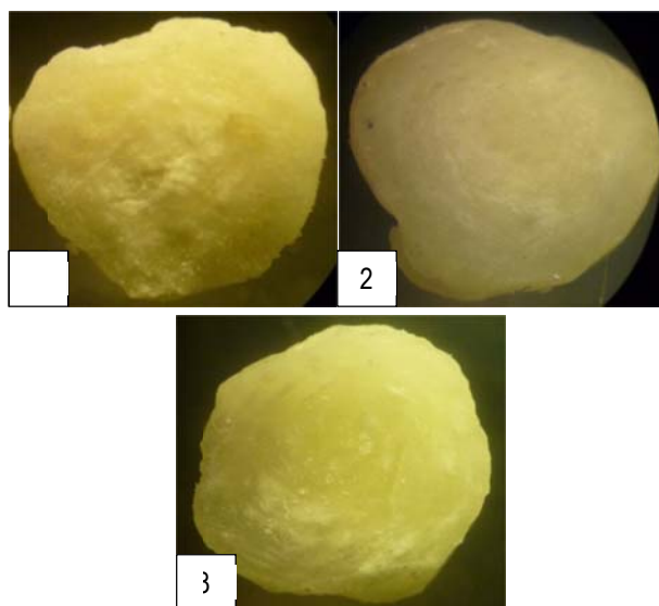
Fig. 5b. Electronic photographs of a granule slice of DAP with different MgO content (magnification \times 25 ) 1 – without adding of MgO (0,12% MgO); 2 – 0,4% MgO; 3 – 0,5% MgO
