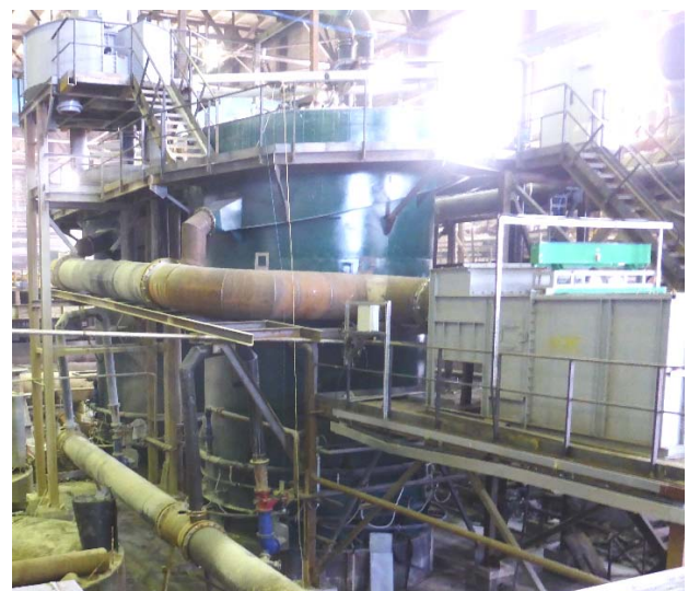
Fig. 3. Re-cleaning of apatite concentrate in the former nepheline concentrate production building at ANOF-2
