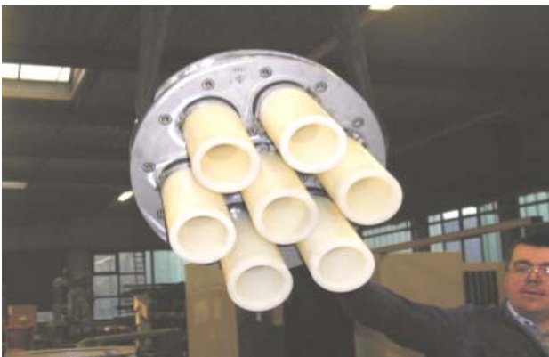
Fig. 2. Imhoflot – aerator in assembly (Imhof, et al., 2005)
