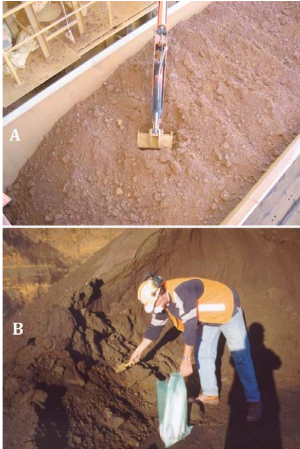
Fig. 2. Taking samples from the top of railway wagons (A) and the side of stockpiles (B) (Morrison et al., 2008)
