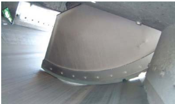
Fig. 5. Cross-belt sample cutter- the conveyor belt profile does not match the trajectory of the cutter (Docherty, 2005; Morrison et al., 2008)
