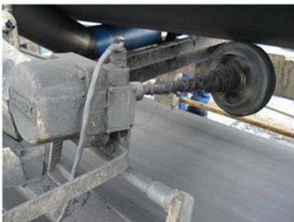
Fig. 7. Tachometer for belt speed measurement (Spangenberg, 2012)
