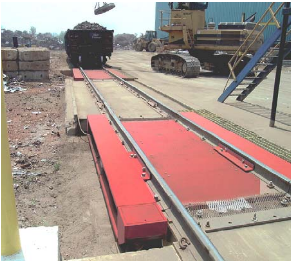
Fig. 2. Railroad track scales (Rice Lake Weighing Systems Ltd.)
