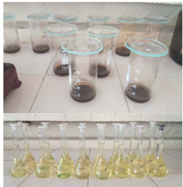
Fig. 9. Preparation of the samples by the method of acid dissolution
