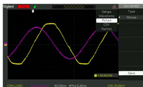
Fig. 12. Input and output signals for the entire filter
