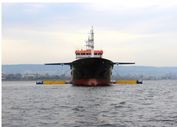
Fig. 19. Oil collection system via sweeping arms
