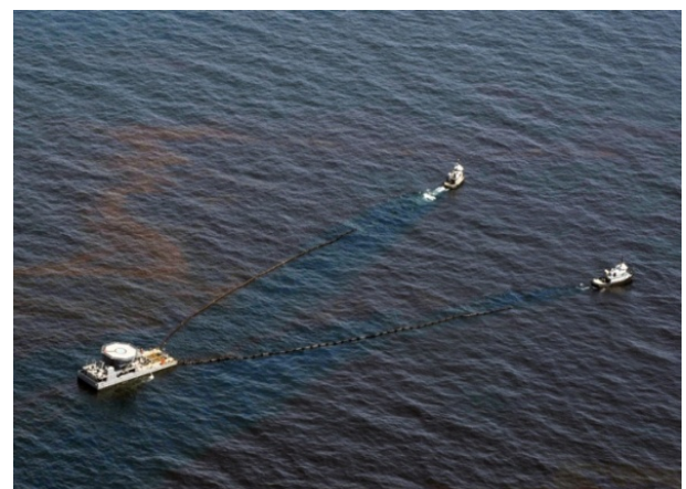
Fig. 16. Offshore oil boom deployed in a "V" configuration (IOGP Report 522, 2015)
