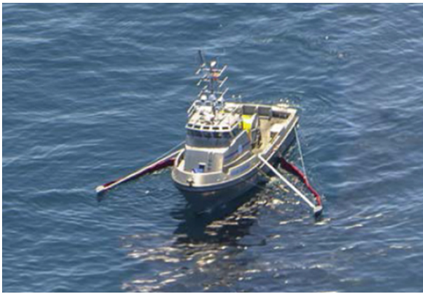
Fig. 17. Single-vessel double-sided oil spill recovery system (IOGP Report 522, 2015)
