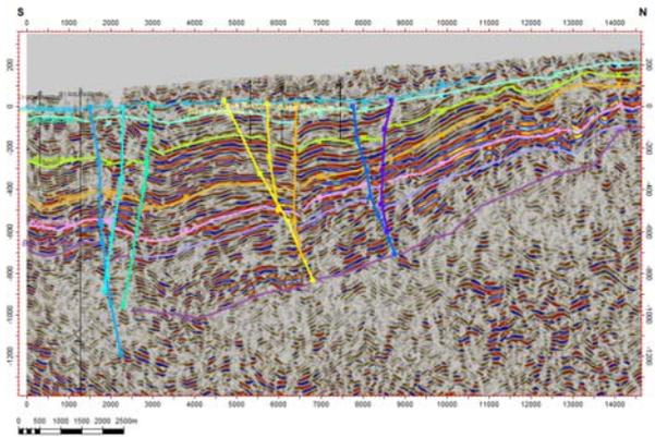
Fig. 3. Geological interpretation of faults and seismic horizons
