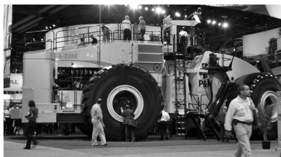
Fig. 10. The Le Torneau P&H L-2350 wheel loader uses a 400 kW SRM
