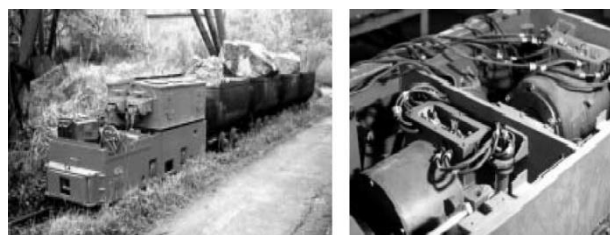
Fig. 8. A mining locomotive with a parallel drive system of two 3-phase SRM6-4
