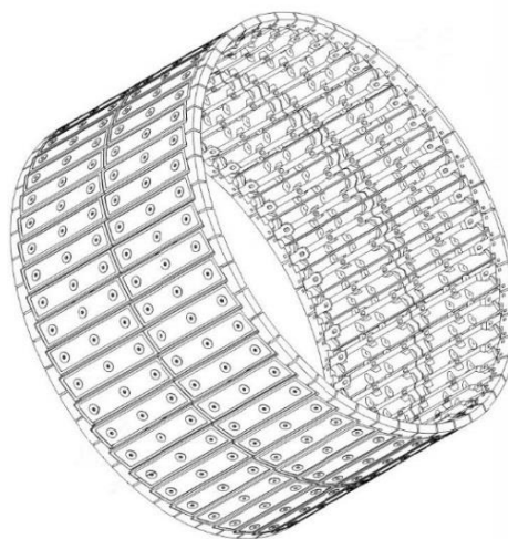
Fig. 1. A linings configuration in a drum SAG mill
