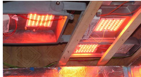
Fig. 10. Cabins № 1 to 5. Lights, each of them emitting in a narrow range of the spectrum
