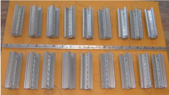
Fig. 5. 18 luminaires, each of which radiates in a narrow area of the visible spectrum
