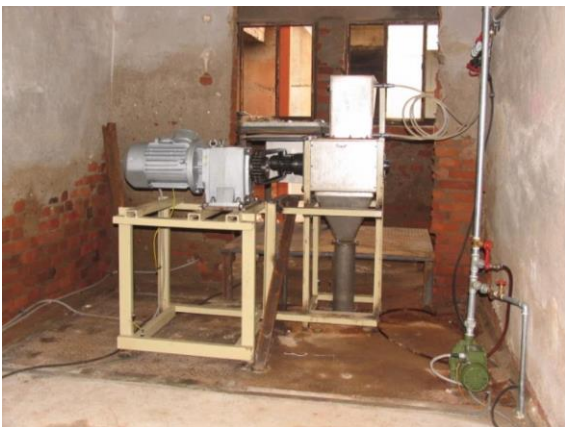
Fig. 3. General appearance of the grinding mill for secondary smokeless gunpowder
