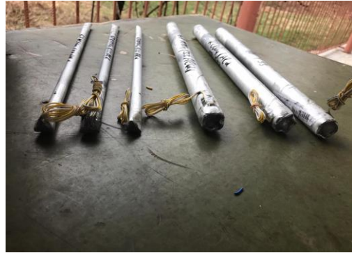
Fig. 4. Loaded and plugged aluminium pipes with el. igniter - ready for test samples
