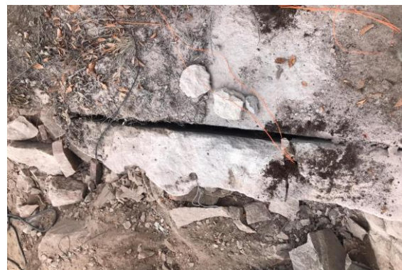
Fig. 9. Effect after experimental cautious blast-splitting of stone slice with divided chain-charges
