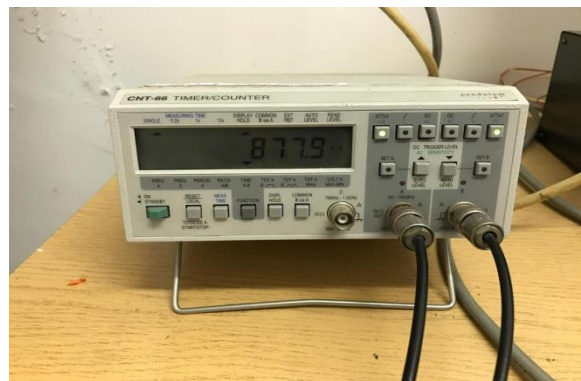
Fig. 6. Apparatus for measurement of VOD with an impact sensor
