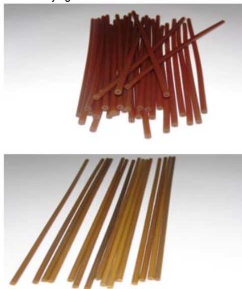
Fig. 1. General image of DBP type NDT-3 18/1 and SBP type 18/1 (down)
