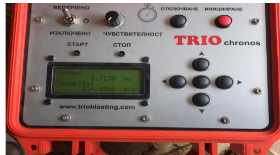
Fig. 5. Apparatus for measurement of VOD optical sensors
