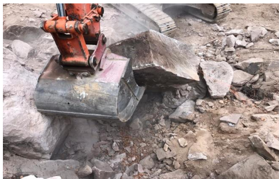
Fig. 11. Results after the experimental blasting with propellant-based non-detonating compositions (Mixtures #2 and #3)
