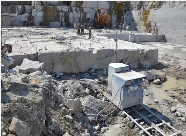
Fig. 4. Implementation of the technology of cutting by disk saw machine at Pokostovsky granite deposit (Ukraine)
