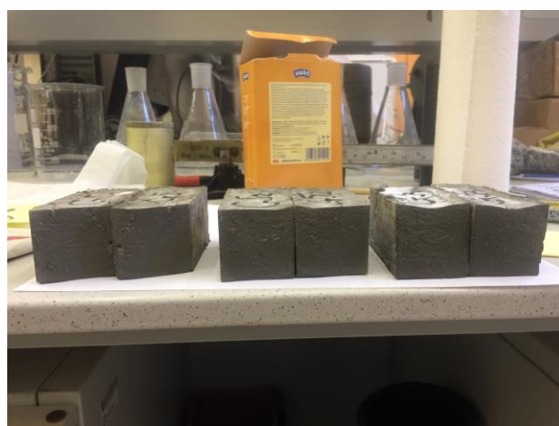
Fig. 2. Samples of cement stone under the influence of different temperatures
