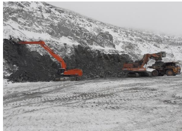
Fig.2. Part of the technological process of bench (sub-bench) formation
