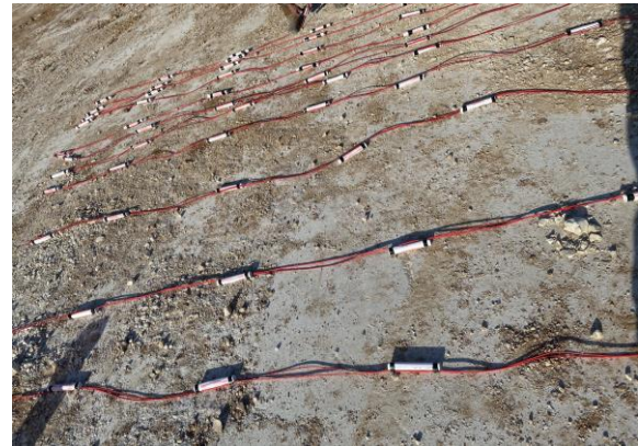
Fig.3. Decoupled multi-deck chained charge loading
