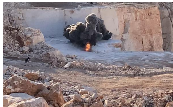
Fig.5. Split-blasting for removal of waste rock close to high quality material
