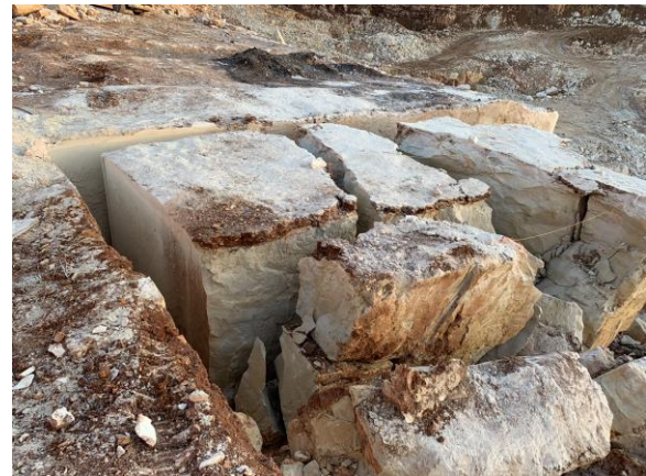
Fig.13. Muckpile of waste rock after blasting of the pre-cutted block
