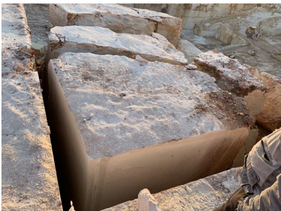
Fig.12. Effect of mechanical pre-cutting
