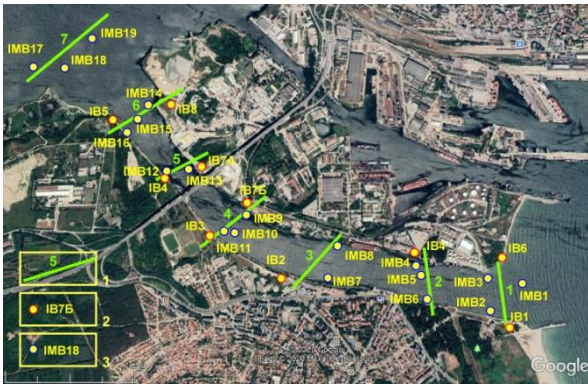
Fig. 2. Satellite map of the borehole profiles across Channel 1: 1, profile; 2, onshore borehole; 3, marine borehole
