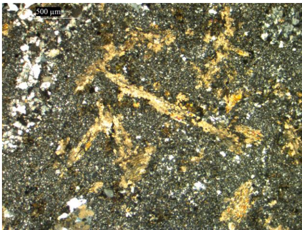
Fig. 4. Altered amphibole crystals with carbonate and chlorite (CPL).
