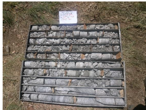
Fig. 1. Typical sequence of intact and crushed core intervals (depth interval 37m-47m).
