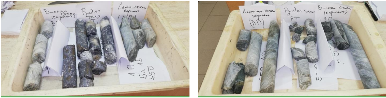
Fig. 3. Grouping of a sets of rock specimens taken from the individual ore bodies in laboratory conditions
