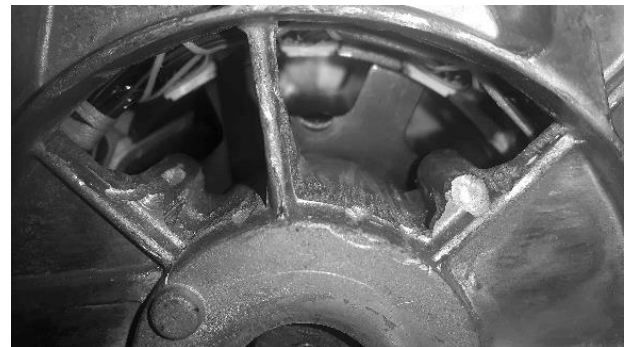
Fig. 8. An opening in the motor housing exposing the salient pole construction of the rotor
