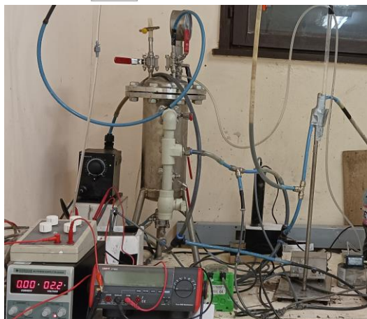
Fig. 1. The technological scheme and photograph of an integrated AD-MEC system.
