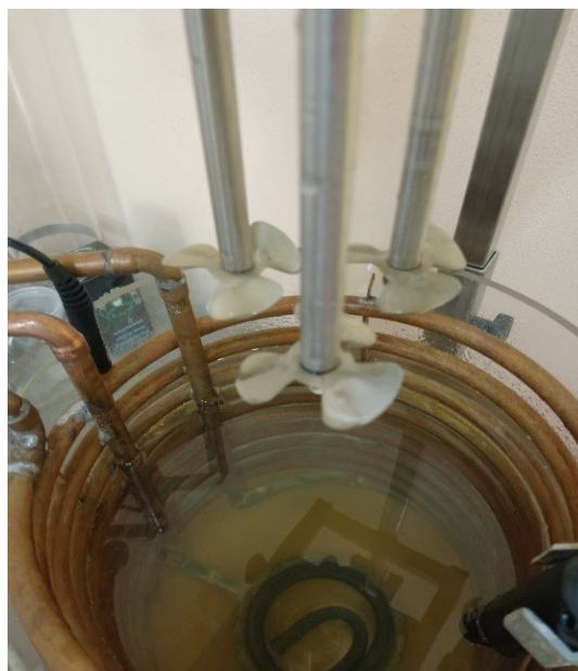
Fig. 1. Picture of the new stirring device with three working bodies.
