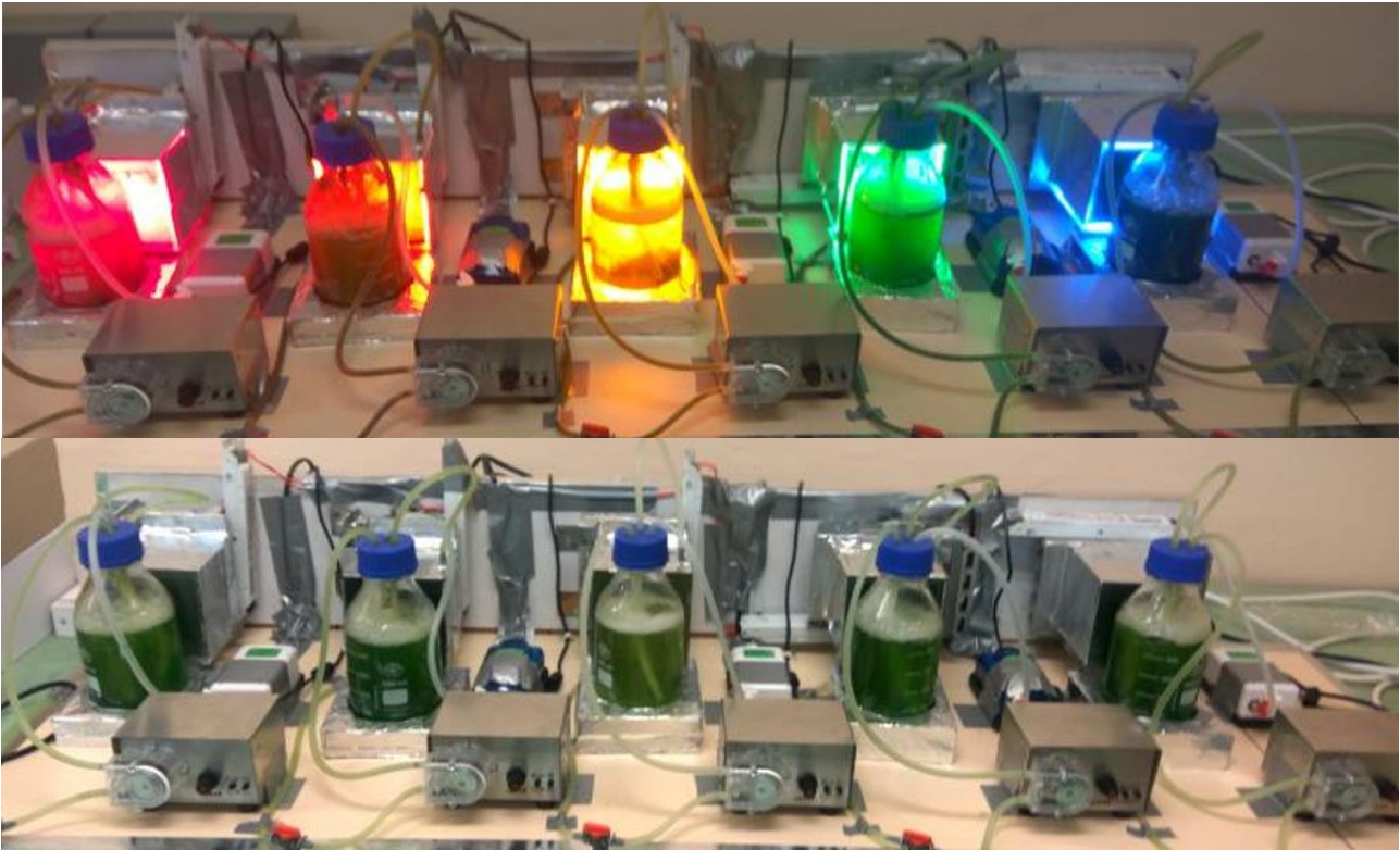
Fig.1. Laboratory installation to research the influence of wavelength on the growth and development of microalgae used in the cathode zone of the MFC.
