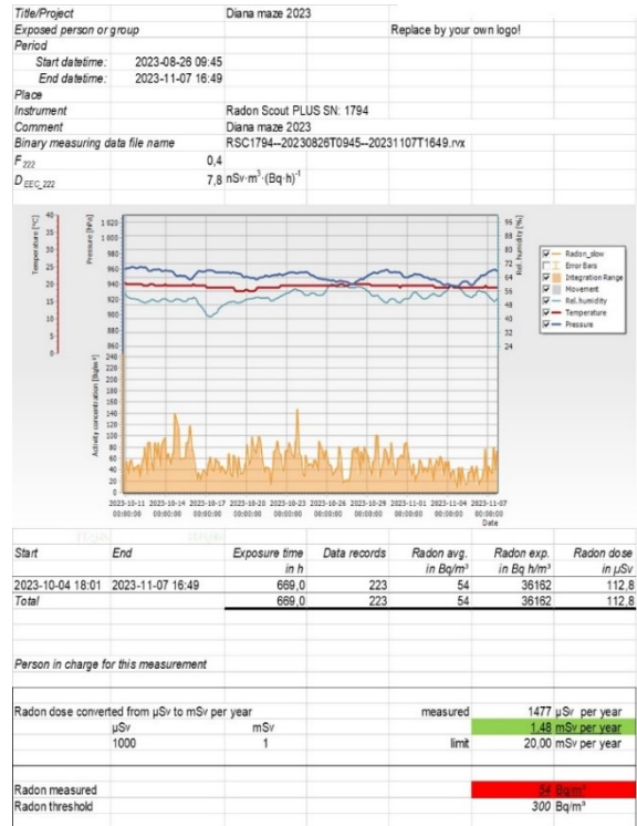
Fig. 15. Radon Scout PLUS measuring report for Object III
