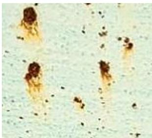
Fig. 14. Pitting corrosion
