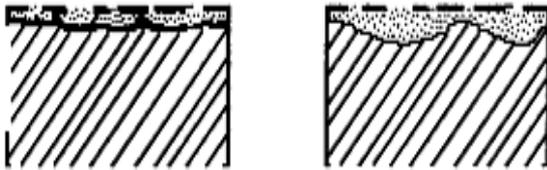
Fig. 12. Schematic of uniform (left) and non-uniform (right) corrosion
