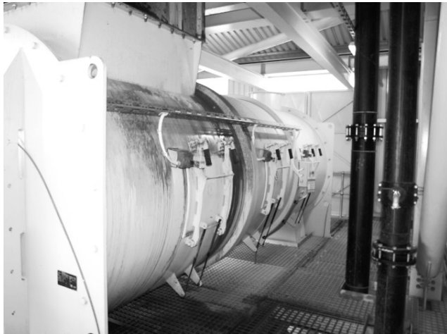
Fig. 6. Mixer for mixing the filtered waste, dry cement, and unfiltered waste
