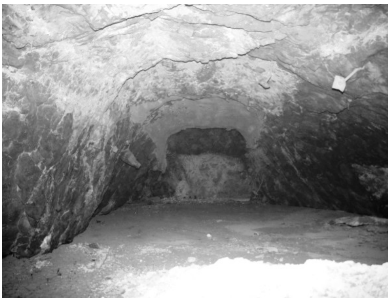
Fig. 2. Surface of a chamber filled with paste fill
