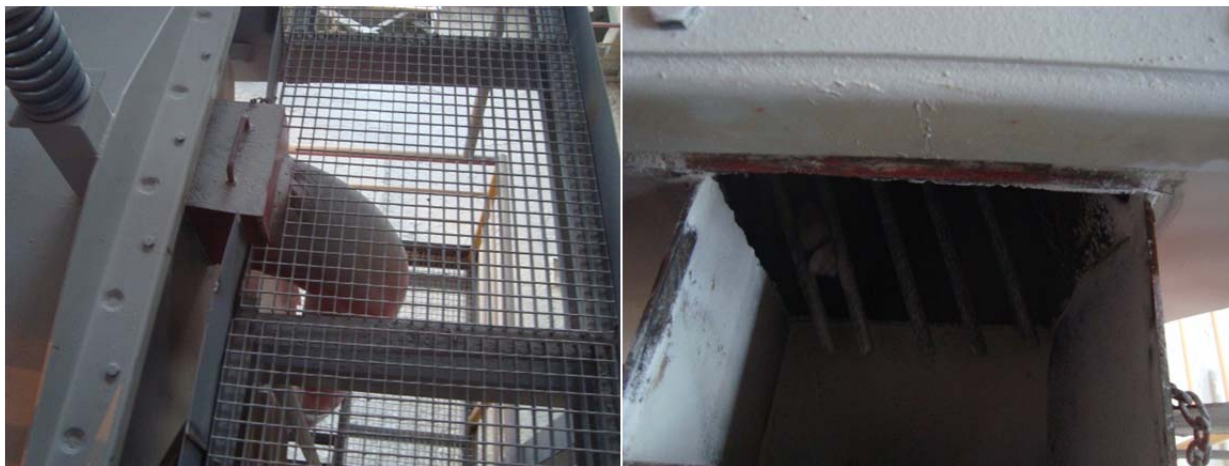
Fig. 9 – Device for lumps removal from vibrating feeder
