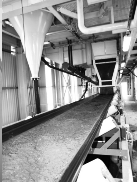
Fig. 5. Belt conveyor for supplying the filtered waste
