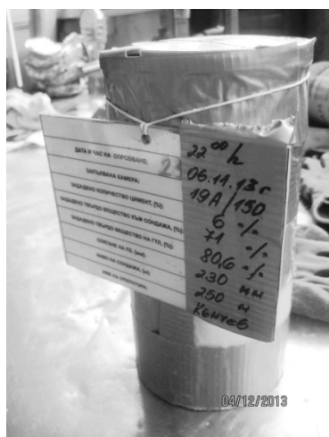
Fig.11. Sample from paste fill tested for uniaxial strength in laboratory conditions
